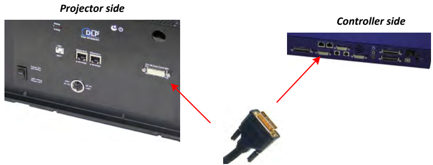
Figure 12 DVI cable between projector and controller
