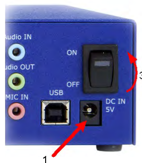
Figure 4 DATAPixx power up procedure
