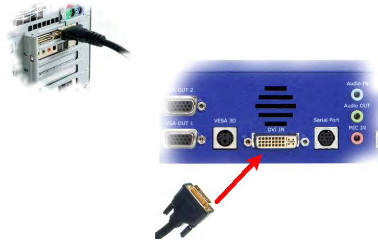
Figure 3 DVI cable between DATAPixx and computer
