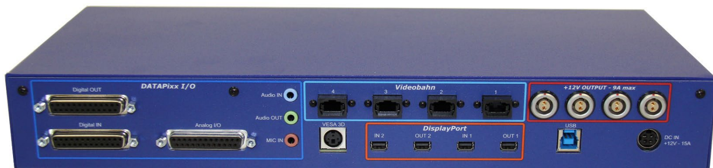
Figure 2 - DATAPixx3 rear panel connectors
