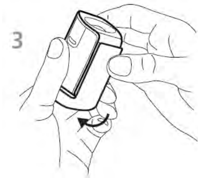
Figure 11 Snapping ambient diffuser arm into place
