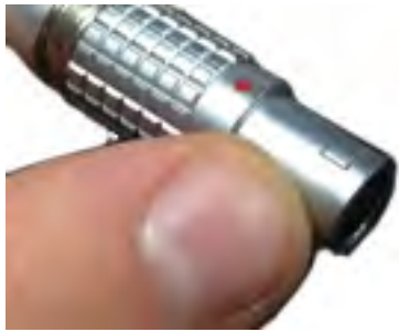
Figure 2 - cable connector red dot and notch
