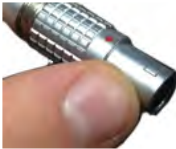
Figure 2 - cable connector red dot and notch
