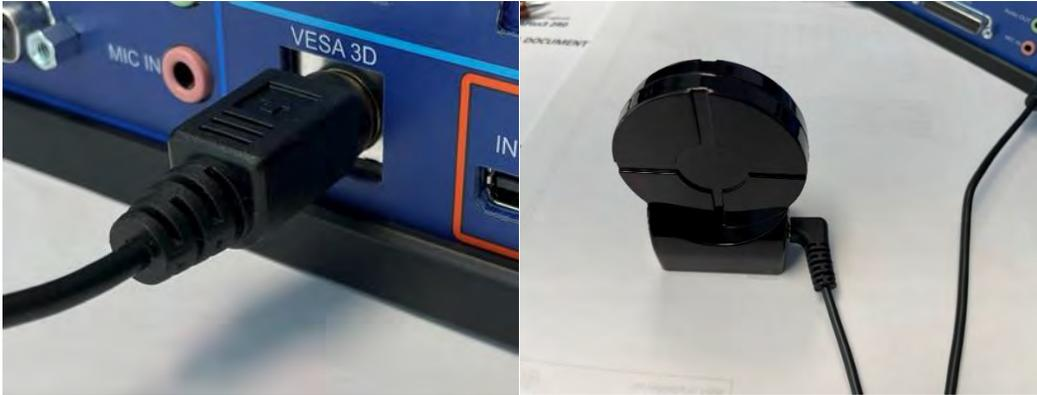
Figure 3. 3DPixx VESA connection and RF Emitter 3D sync input
